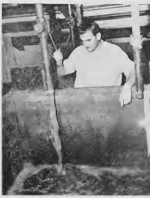
Aloé juice is charged into one of the tanks which separate out the plant resin and other impurities. After further chemical processing, the pure aloin is dried and dried in a large oven.
